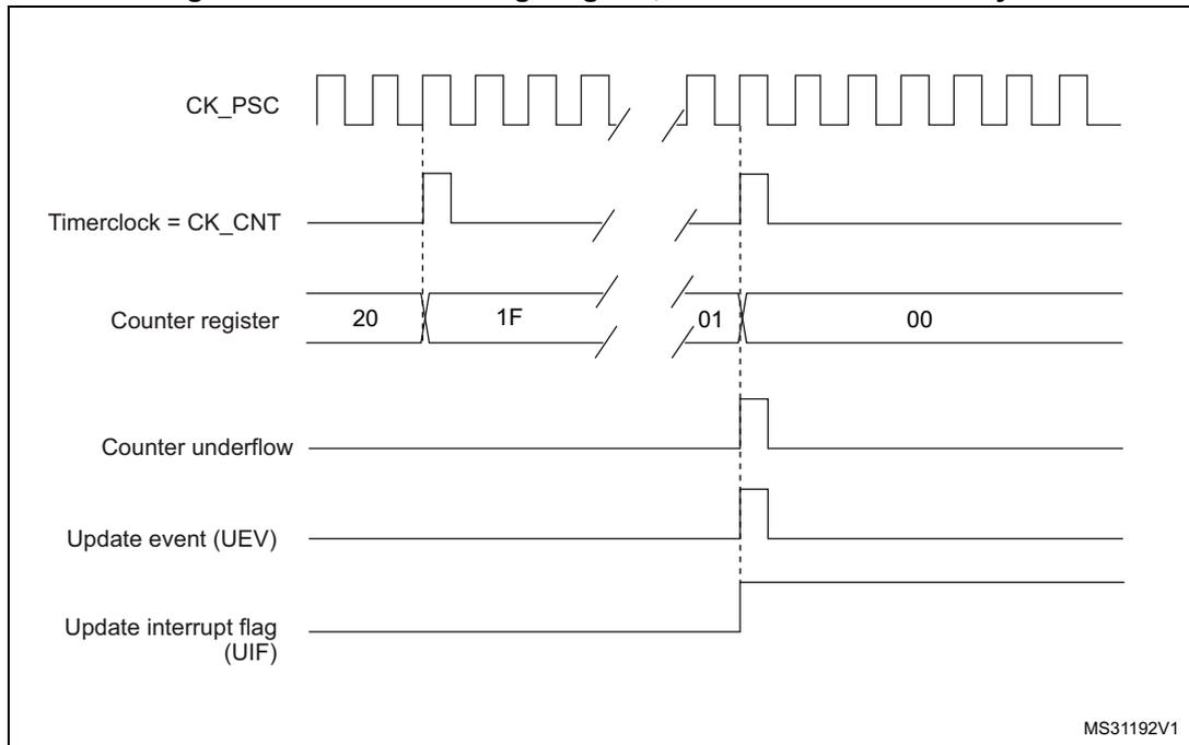
**Figure 140. Counter timing diagram, Update event with ARPE=1 (counter underflow)**
