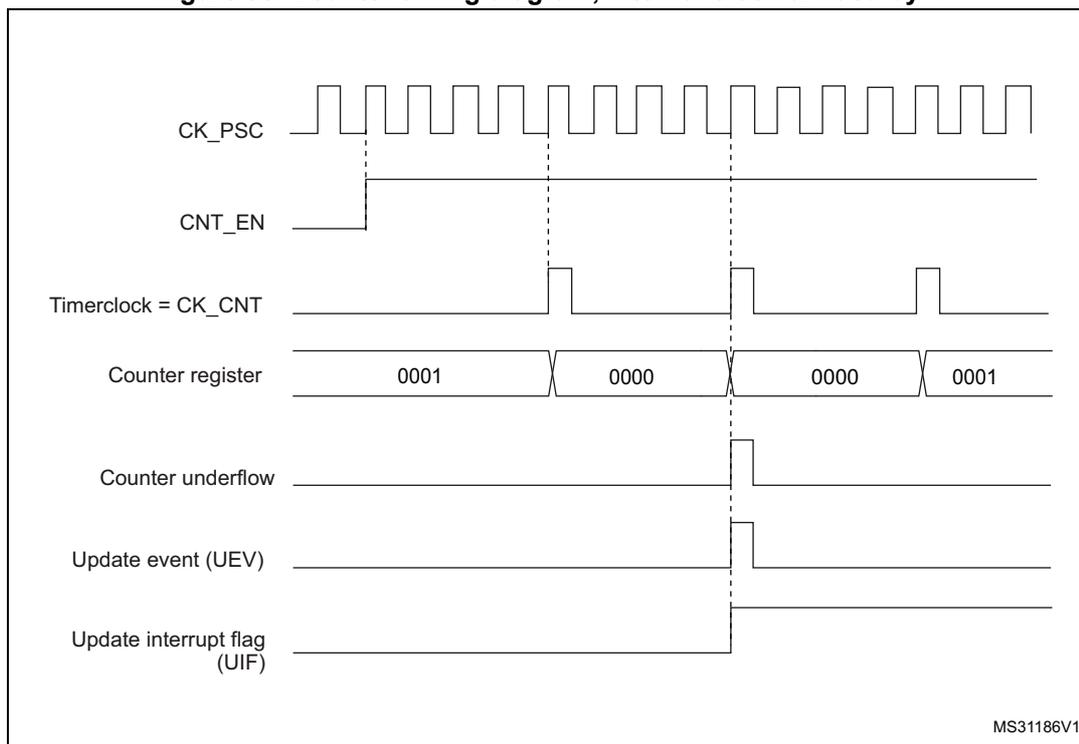
Figure 89. Counter timing diagram, internal clock divided by N
