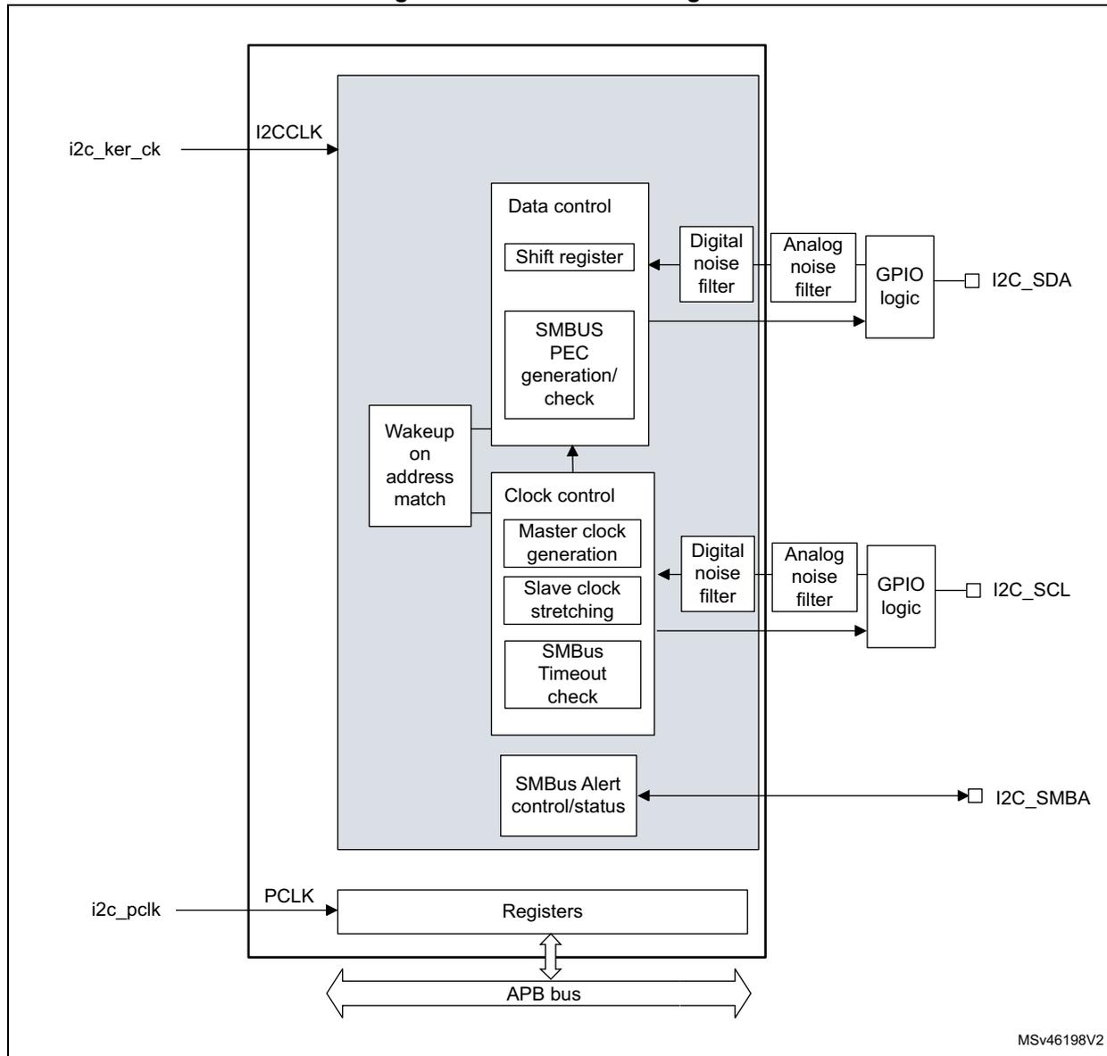
The I2C1/3 is clocked by an independent clock source which allows the I2C to operate independently from the PCLK frequency.
