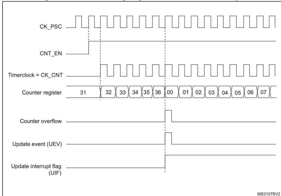
**Figure 127. Counter timing diagram, internal clock divided by 2**
