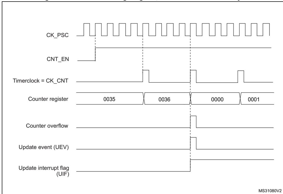
Figure 167. Counter timing diagram, internal clock divided by N
