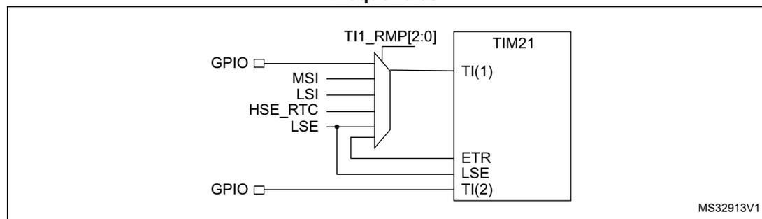
TIM21 has an input multiplexer that selects which of the I/O or the internal clock is to trigger the input capture. This selection is performed through the T11\_RMP [2:0] bits in the TIM21\_OR register.
