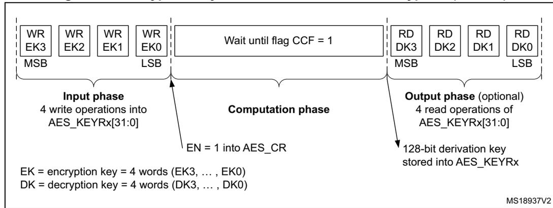
If the software stores the initial key prepared for decryption, it is enough to do the key schedule operation only once for all the data to be decrypted with a given cipher key.
