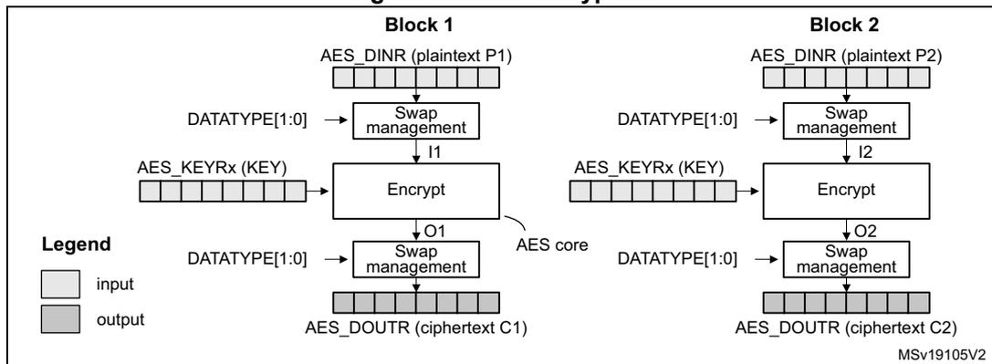
In ECB encrypt mode, the 128-bit plaintext input data block P<sub>x</sub> in the AES\_DINR register first goes through bit/byte/half-word swapping. The swap result I<sub>x</sub> is processed with the AES core set in encrypt mode, using a 128-bit key. The encryption result O<sub>x</sub> goes through bit/byte/half-word swapping, then is stored in the AES\_DOUTR register as 128-bit ciphertext
