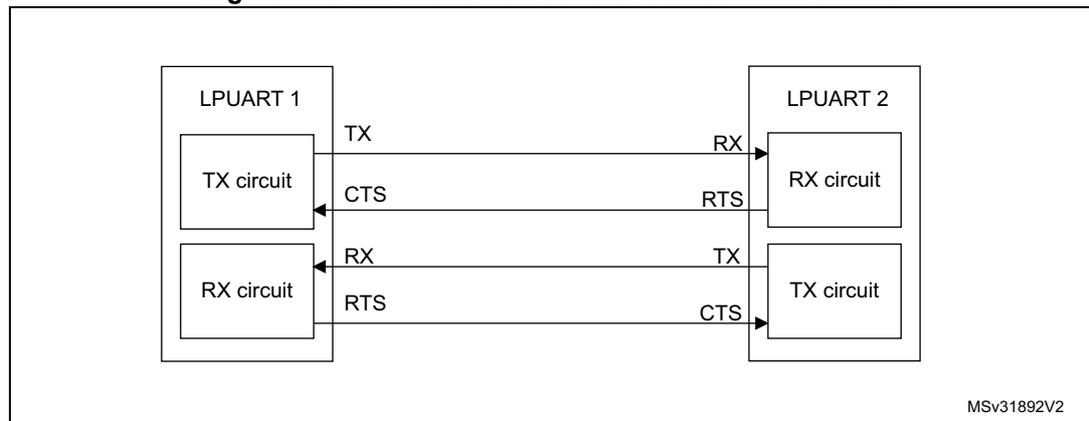
RS232 RTS and CTS flow control can be enabled independently by writing the RTSE and CTSE bits respectively to 1 (in the LPUART\_CR3 register).
