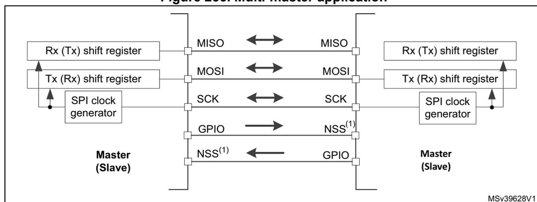
1. The NSS pin is configured at hardware input mode at both nodes. Its active level enables the MISO line output control as the passive node is configured as a slave.
