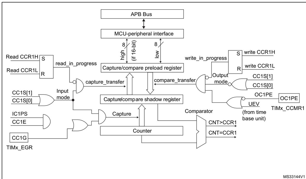
Figure 104. Output stage of capture/compare channel (channel 1)
