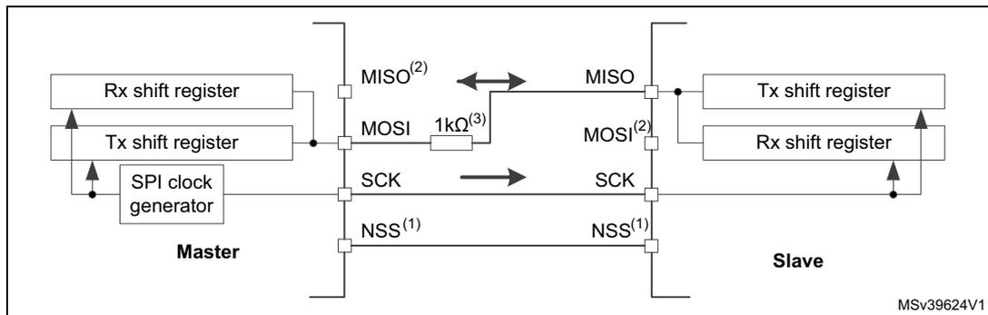
1. The NSS pins can be used to provide a hardware control flow between master and slave. Optionally, the pins can be left unused by the peripheral. Then the flow has to be handled internally for both master and slave. For more details see [Section 26.3.5: Slave select \(NSS\) pin management](#).
