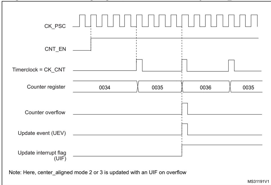
1. Center-aligned mode 2 or 3 is used with an UIF on overflow.
