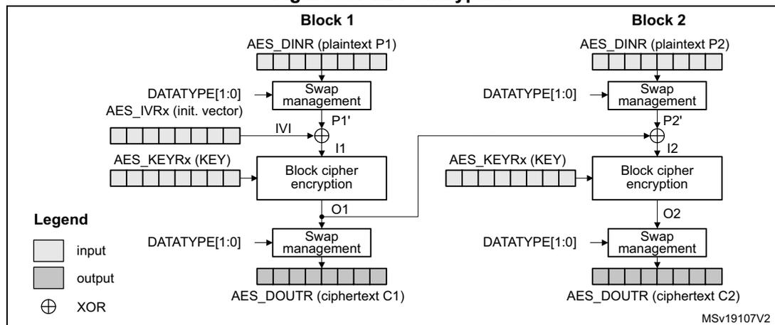
In CBC encrypt mode, the first plaintext input block, after bit/byte/half-word swapping (P1'), is XOR-ed with a 128-bit IVI bitfield (initialization vector and counter), producing the I1 input data for encrypt with the AES core, using a 128- key. The resulting 128-bit output block O1, after swapping operation, is used as ciphertext C1. The O1 data is then XOR-ed with the
