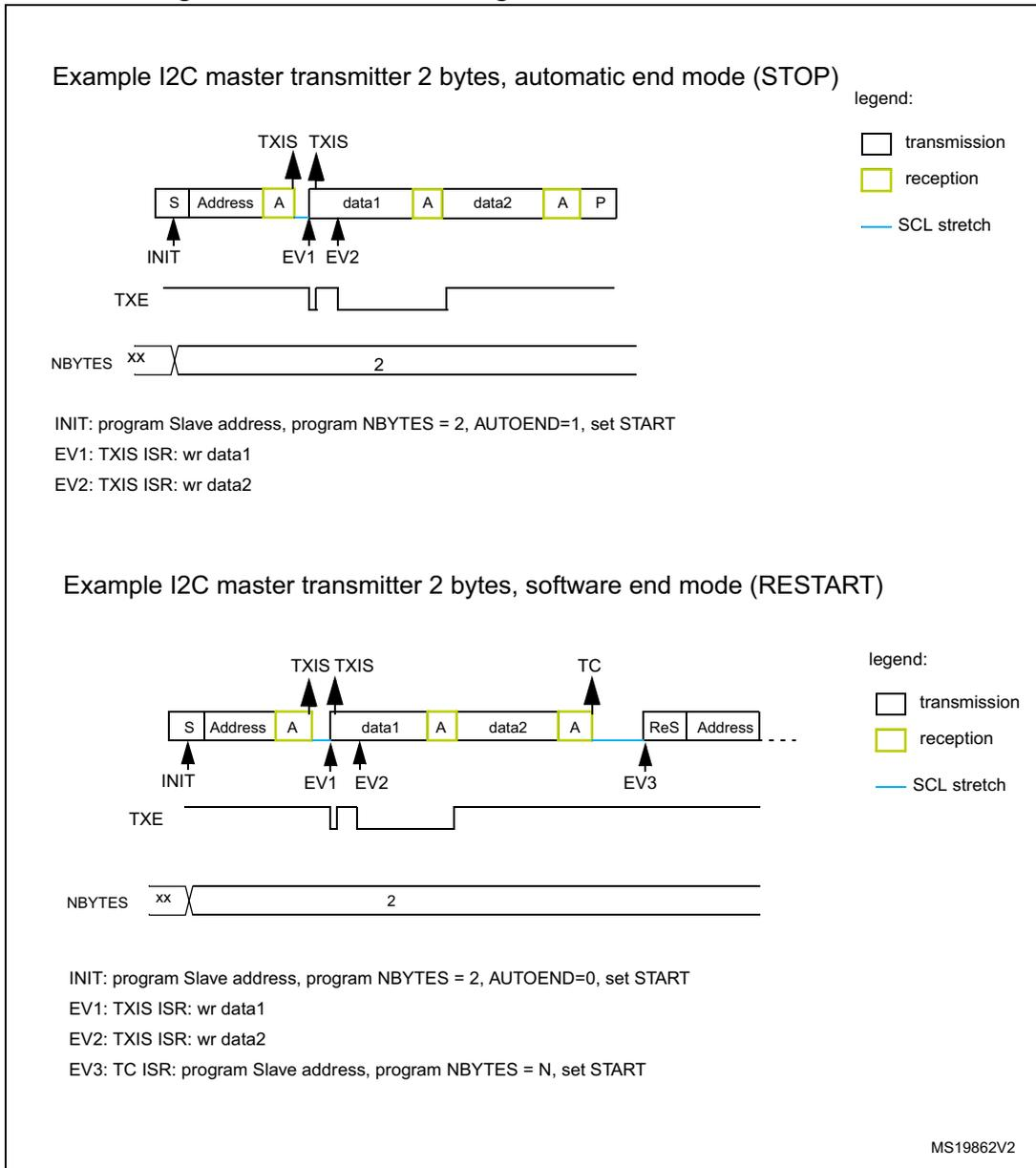
For code example, refer to [A.14.6: I2C master transmitter code example](#).
