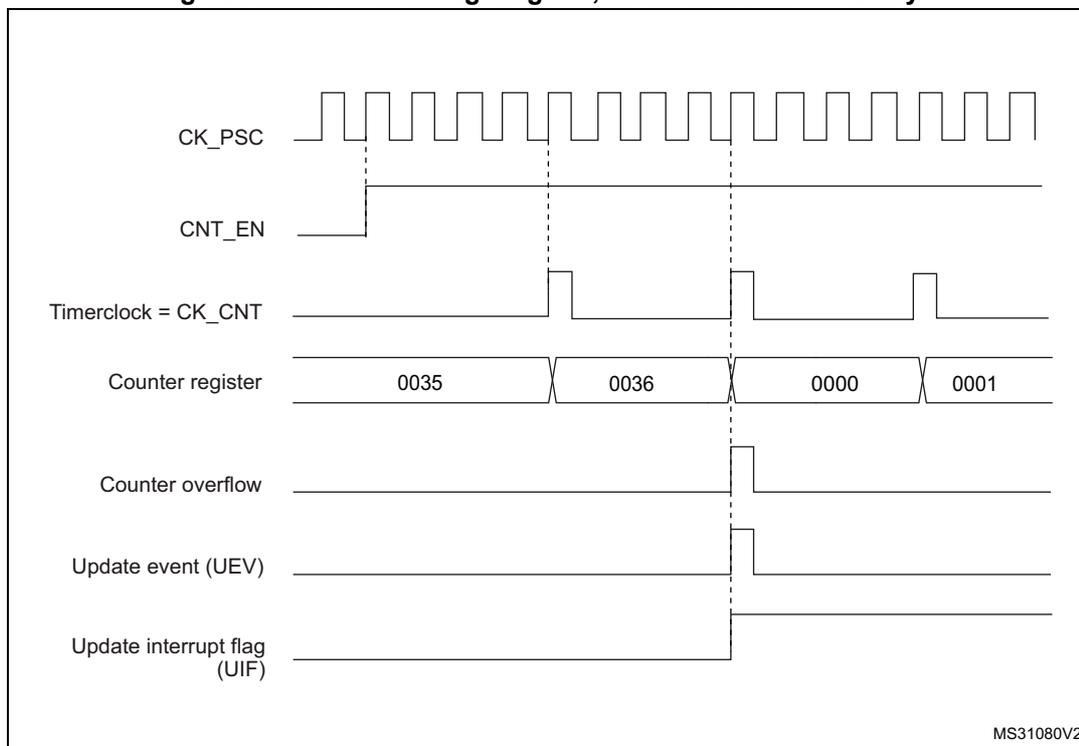
Figure 83. Counter timing diagram, internal clock divided by N
