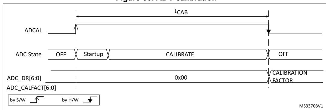
If the ADC voltage regulator was not previously set, it is automatically enabled when setting ADCAL = 1 (bit ADVREGEN is automatically set by hardware). In this case, the ADC calibration time is longer to take into account the stabilization time of the ADC voltage regulator.
