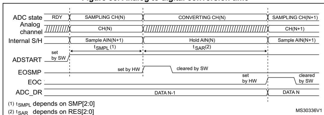
Figure 36. ADC conversion timings
