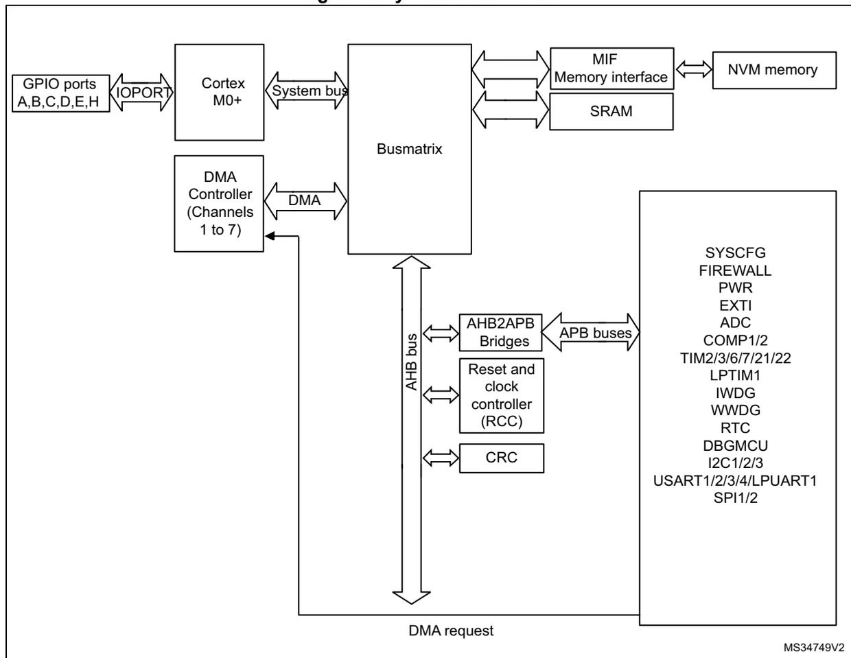
1. Refer to [Table 1: STM32L0x1 memory density](#), to [Table 2: Overview of features per category](#) and to the device datasheets for the GPIO ports and peripherals available on your device.
