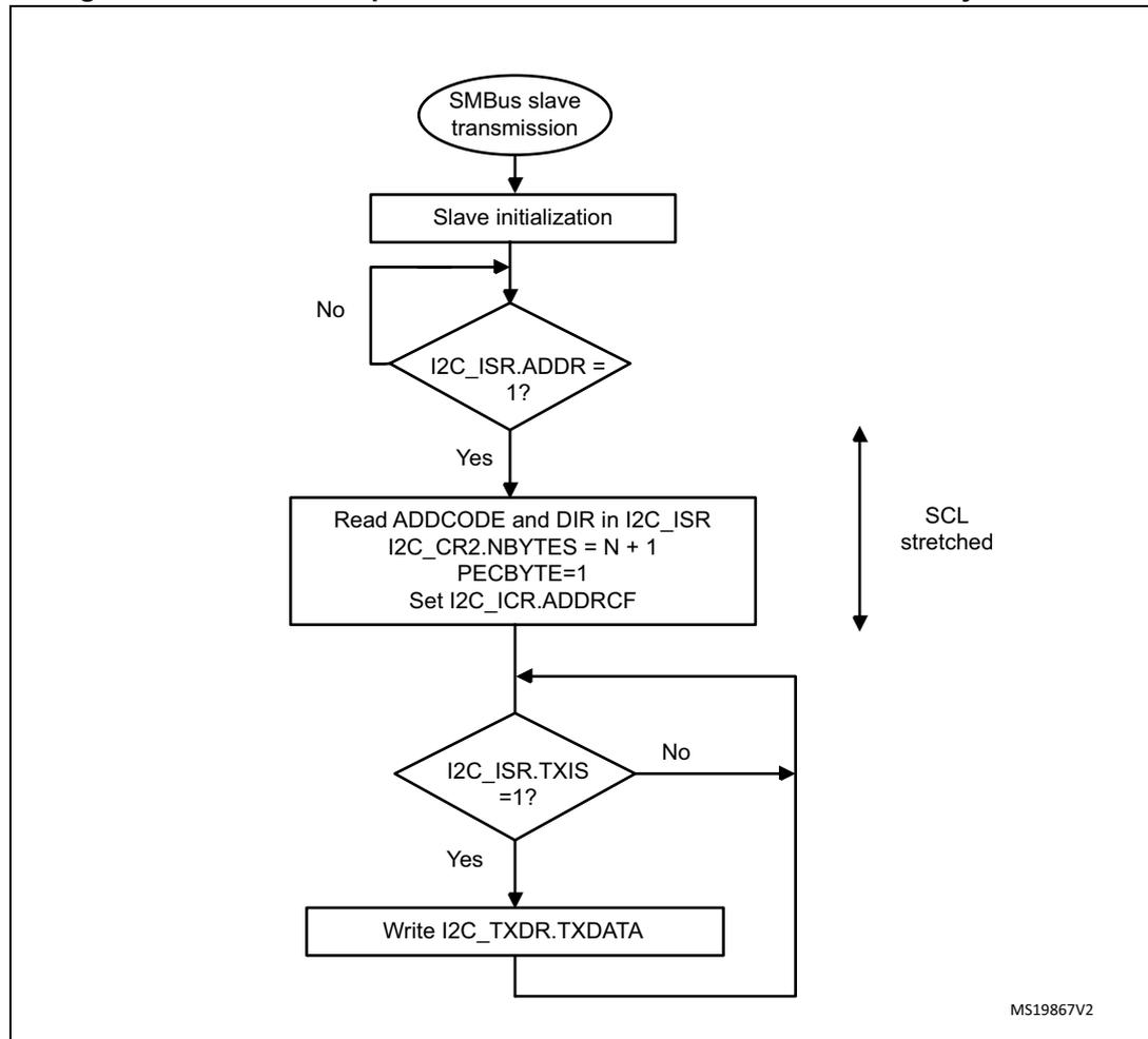
**Figure 208. Transfer bus diagrams for SMBus slave transmitter (SBC=1)**
