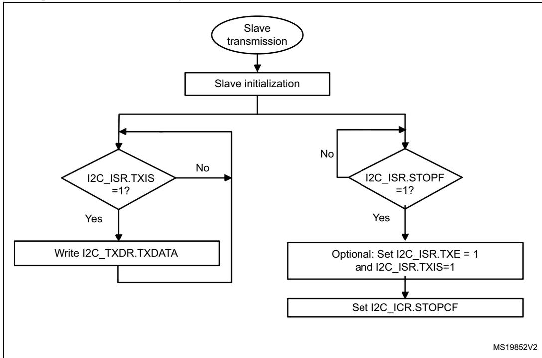
Figure 192. Transfer bus diagrams for I2C slave transmitter
