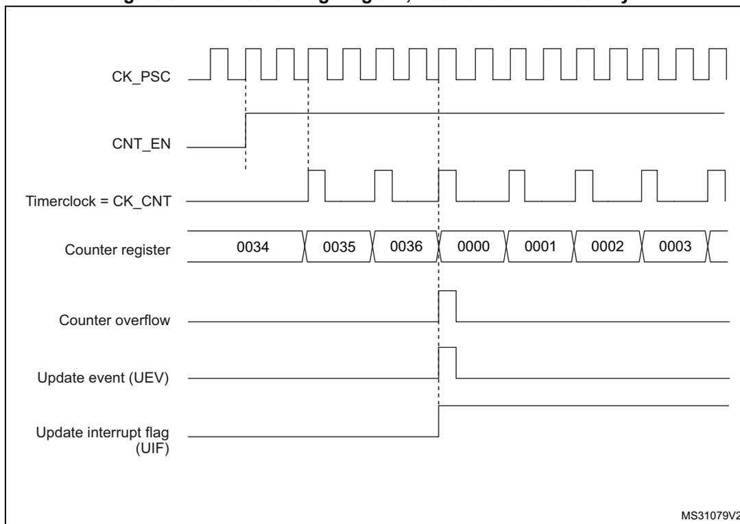
Figure 82. Counter timing diagram, internal clock divided by 4
