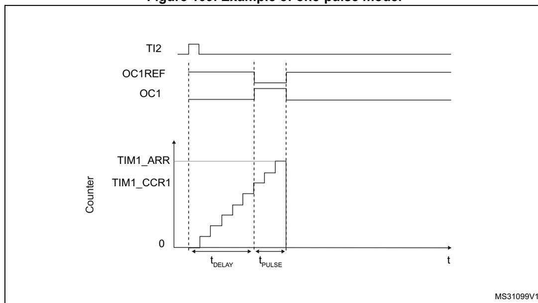
For example one may want to generate a positive pulse on OC1 with a length of  $t_{PULSE}$  and after a delay of  $t_{DELAY}$  as soon as a positive edge is detected on the TI2 input pin.
