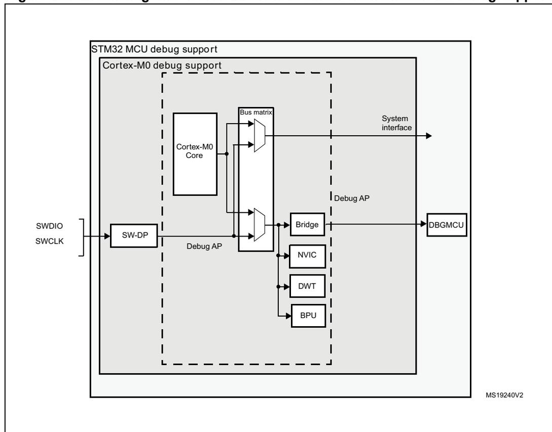
1. The debug features embedded in the Cortex<sup>®</sup>-M0+ core are a subset of the Arm<sup>®</sup> CoreSight Design Kit.
