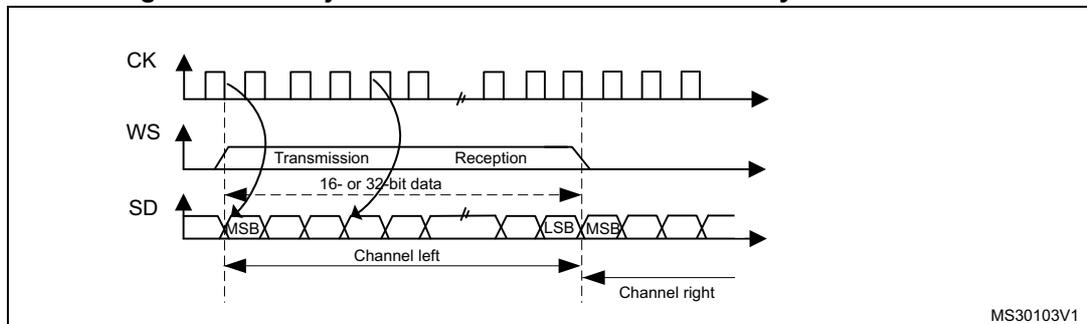
**Figure 275. LSB justified 24-bit frame length with CPOL = 0**
