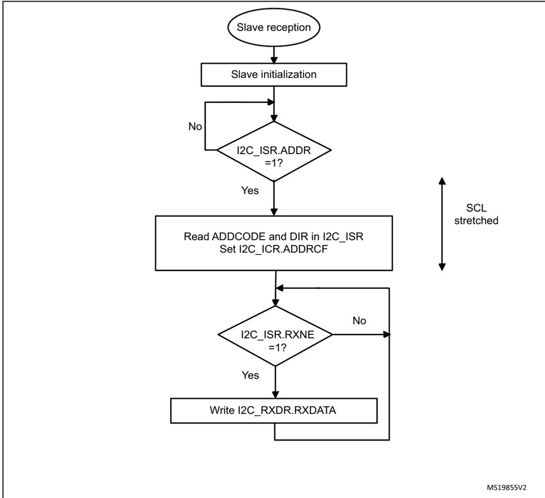
Figure 194. Transfer sequence flow for slave receiver with NOSTRETCH = 1
