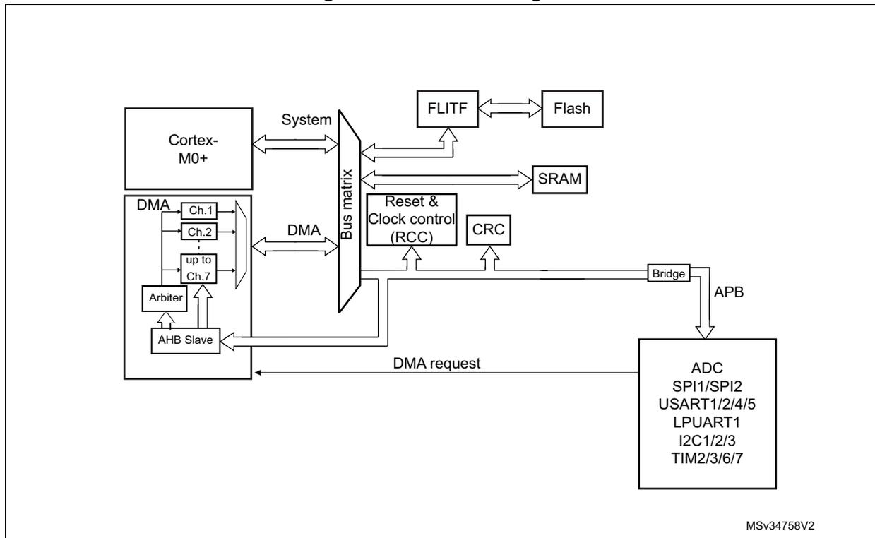
The DMA controller performs direct memory transfer by sharing the AHB system bus with other system masters. The bus matrix implements round-robin scheduling. DMA requests may stop the CPU access to the system bus for a number of bus cycles, when CPU and DMA target the same destination (memory or peripheral).
