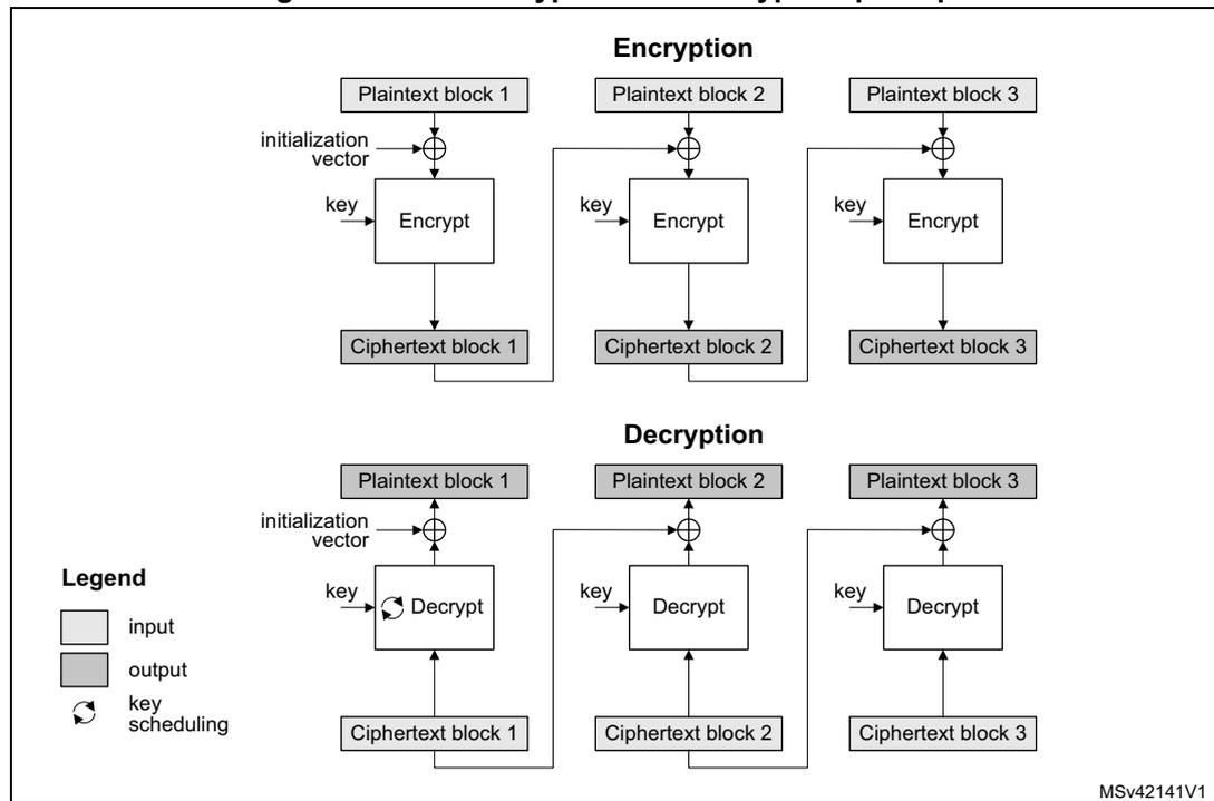
In CBC mode the output of each block chains with the input of the following block. To make each message unique, an initialization vector is used during the first block processing.
