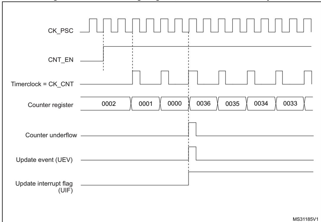
Figure 88. Counter timing diagram, internal clock divided by 4
