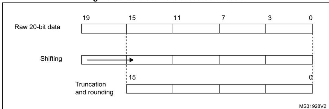
The Figure 53 gives a numerical example of the processing, from a raw 20-bit accumulated data to the final 16-bit result.
