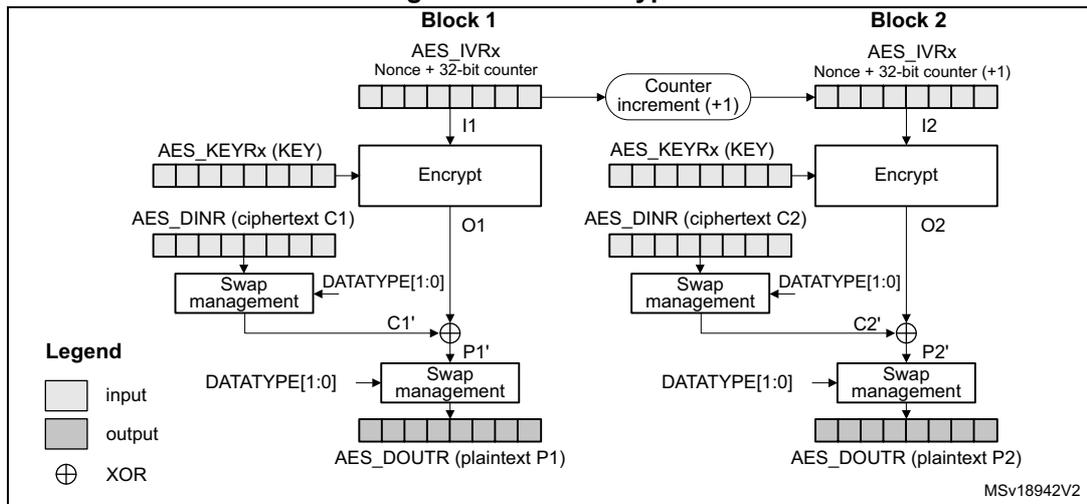
In CTR mode, the cryptographic core output (also called keystream)  $Ox$  is XOR-ed with relevant input block ( $Px'$  for encryption,  $Cx'$  for decryption), to produce the correct output block ( $Cx'$  for encryption,  $Px'$  for decryption). Initialization vectors in AES must be initialized as shown in [Table 69](#).
