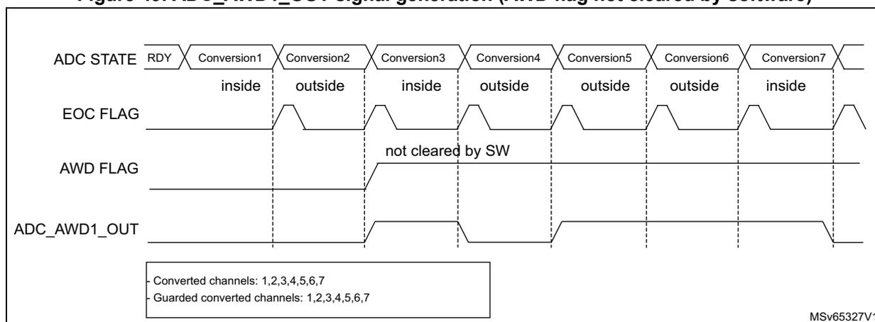
Figure 50. ADC1\_AWD\_OUT signal generation (on a single channel)
