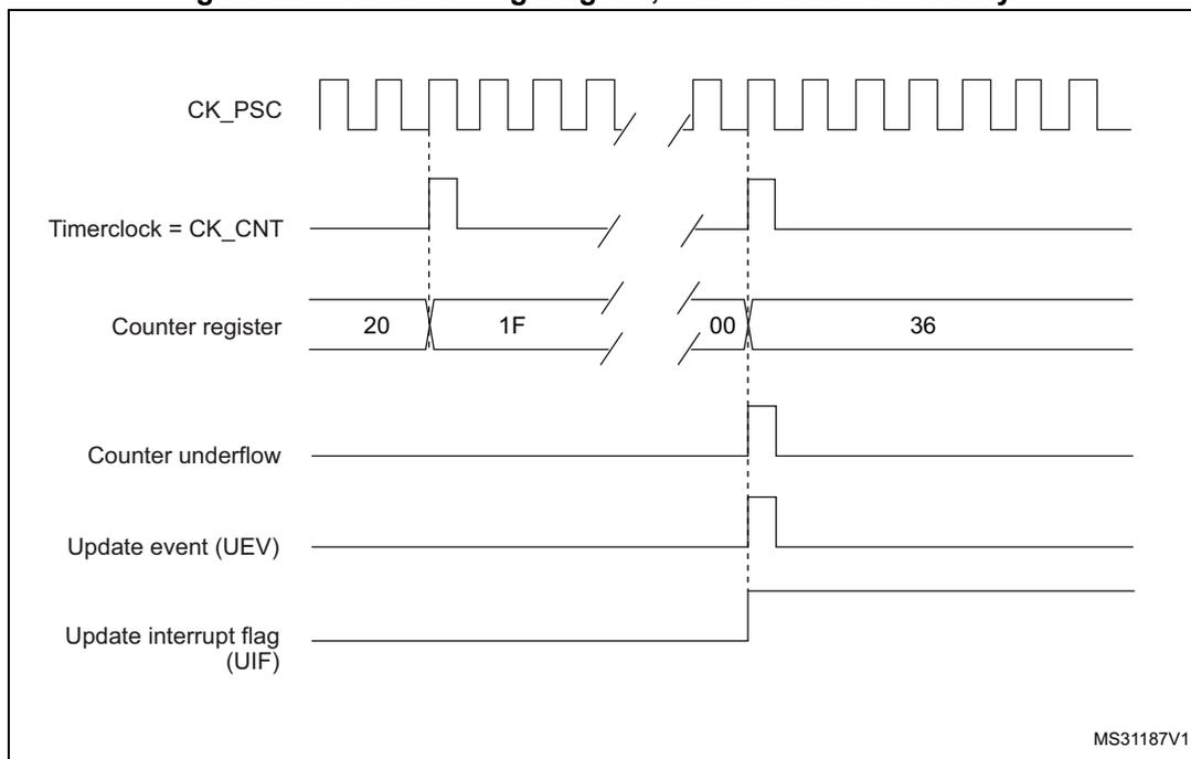
**Figure 90. Counter timing diagram, Update event when repetition counter is not used**
