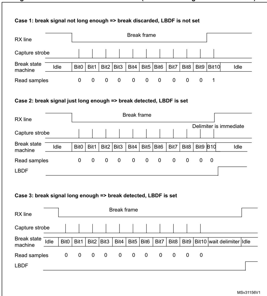
Figure 223. Break detection in LIN mode vs. Framing error detection
