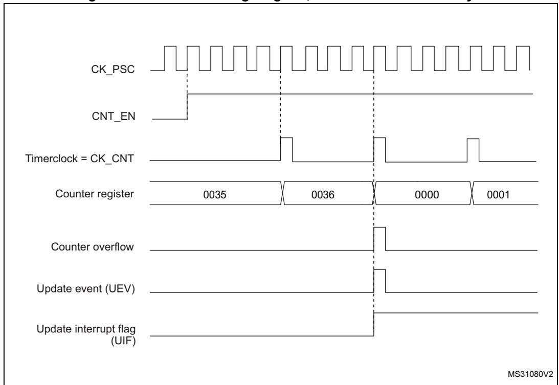
Figure 129. Counter timing diagram, internal clock divided by N
