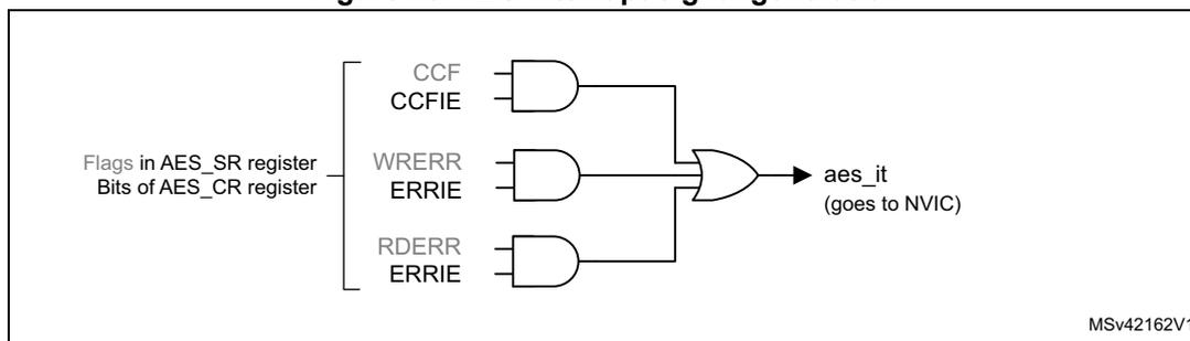
Each AES interrupt source can individually be enabled/disabled, by setting/clearing the corresponding enable bit of the AES\_CR register. See [Figure 76](#).
