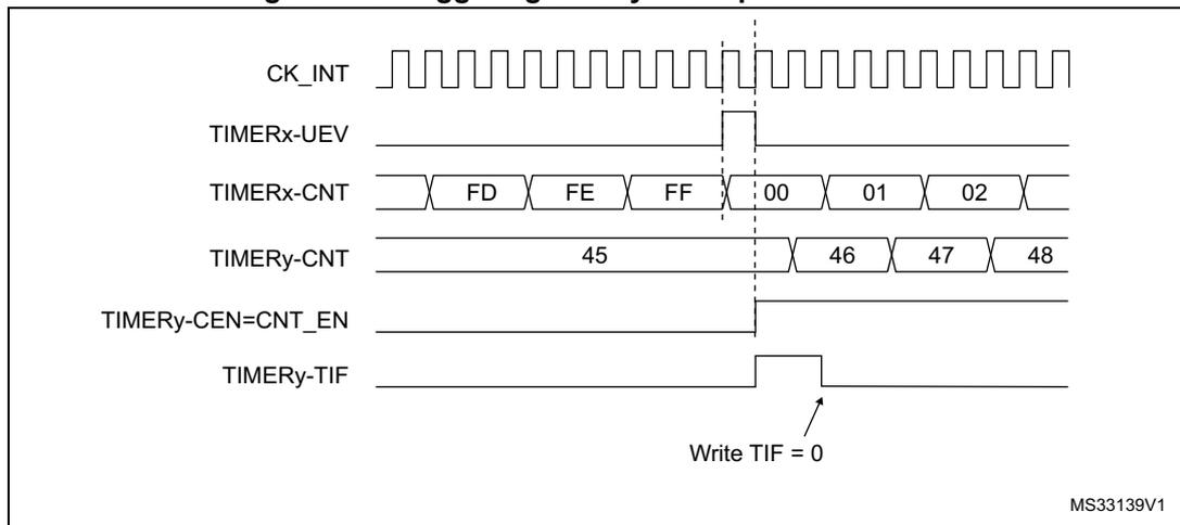
As in the previous example, both counters can be initialized before starting counting. [Figure 121](#) shows the behavior with the same configuration as in [Figure 120](#) but in trigger mode instead of gated mode (SMS=110 in the TIMy\_SMCR register).
