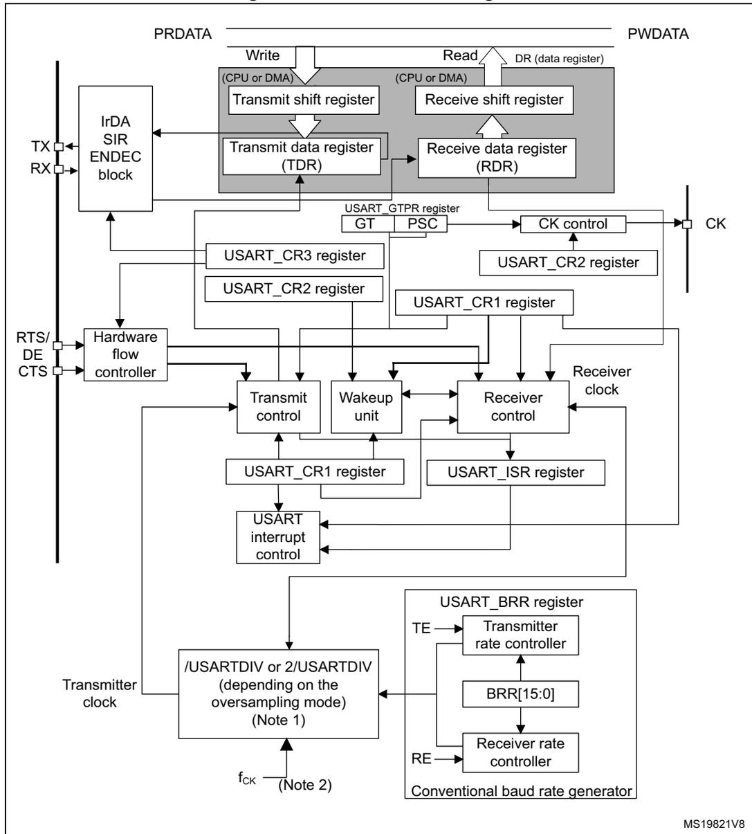
1. For details on coding USARTDIV in the USART\_BRR register, refer to [Section 24.5.4: USART baud rate generation](#).
