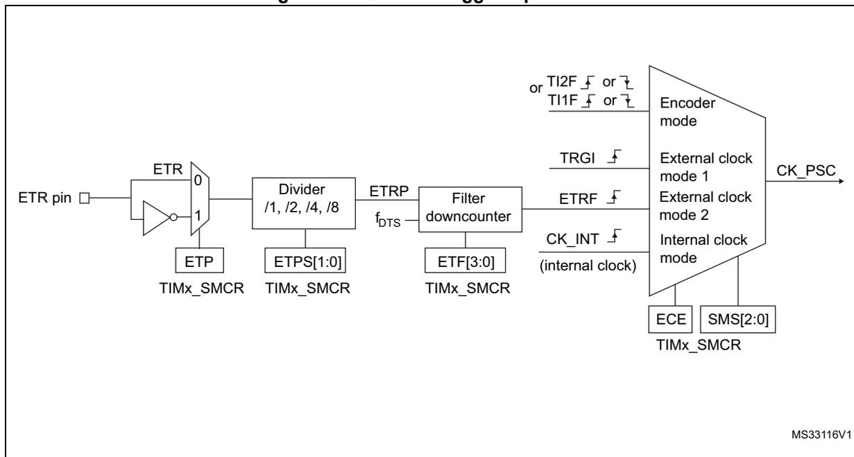
For example, to configure the upcounter to count each 2 rising edges on ETR, use the following procedure:
