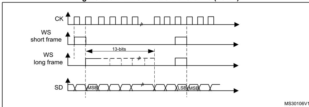
For long frame synchronization, the WS signal assertion time is fixed to 13 bits in master mode.
