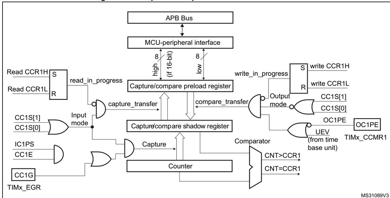
Figure 149. Output stage of capture/compare channel (channel 1 and 2)
