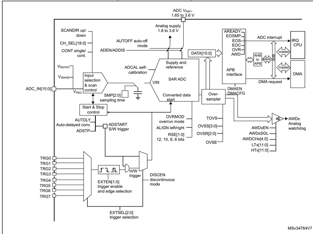
1. TRGi are mapped at product level. Refer to Table External triggers in Section 13.3.1: ADC pins and internal signals.
