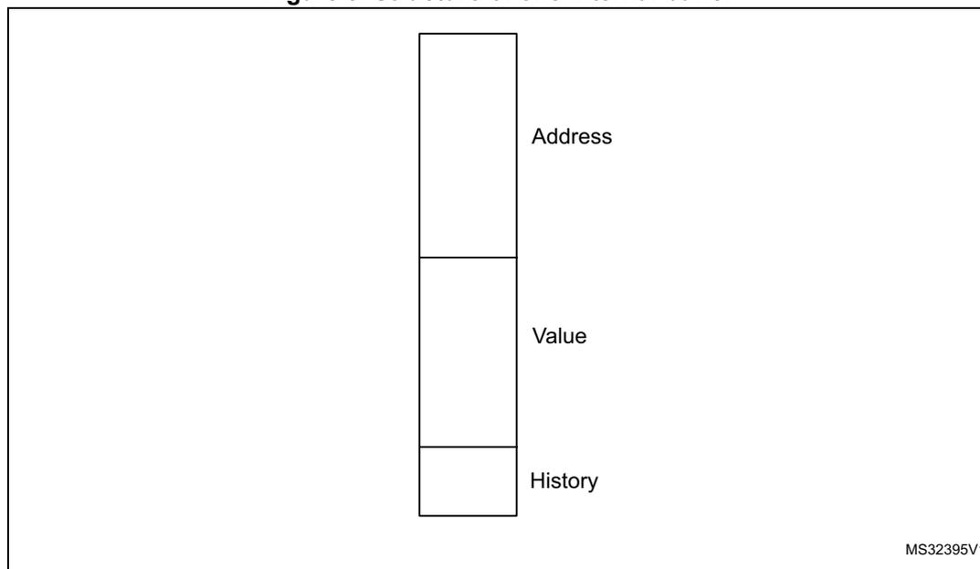
Each buffer stores 3 different types of information: address, data and history. In a read operation, if the address is found, the memory interface can return data without accessing the NVM. Data in the buffer is 32 bit wide (even if the master only reads 8 or 16 bits), so that a value can be returned whatever the size used in a previous reading. The history is used to know if the content of a buffer is valid and to delete (with a new value) the older one.
