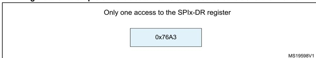
In transmission mode, when a TXE event occurs, the application has to write the data to be transmitted (in this case 0x76A3). The 0x000 field is transmitted first (extension on 32-bit). The TXE flag is set again as soon as the effective data (0x76A3) is sent on SD.
