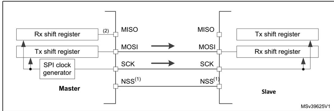
1. The NSS pins can be used to provide a hardware control flow between master and slave. Optionally, the pins can be left unused by the peripheral. Then the flow has to be handled internally for both master and slave. For more details see [Section 26.3.5: Slave select \(NSS\) pin management](#).
