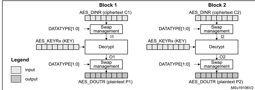
To perform an AES decryption in the ECB mode, the secret key has to be prepared by collecting the last-round encryption key (which requires to first execute the complete key schedule for encryption), and using it as the first-round key for the decryption of the ciphertext. This preparation is supported by the AES core.
