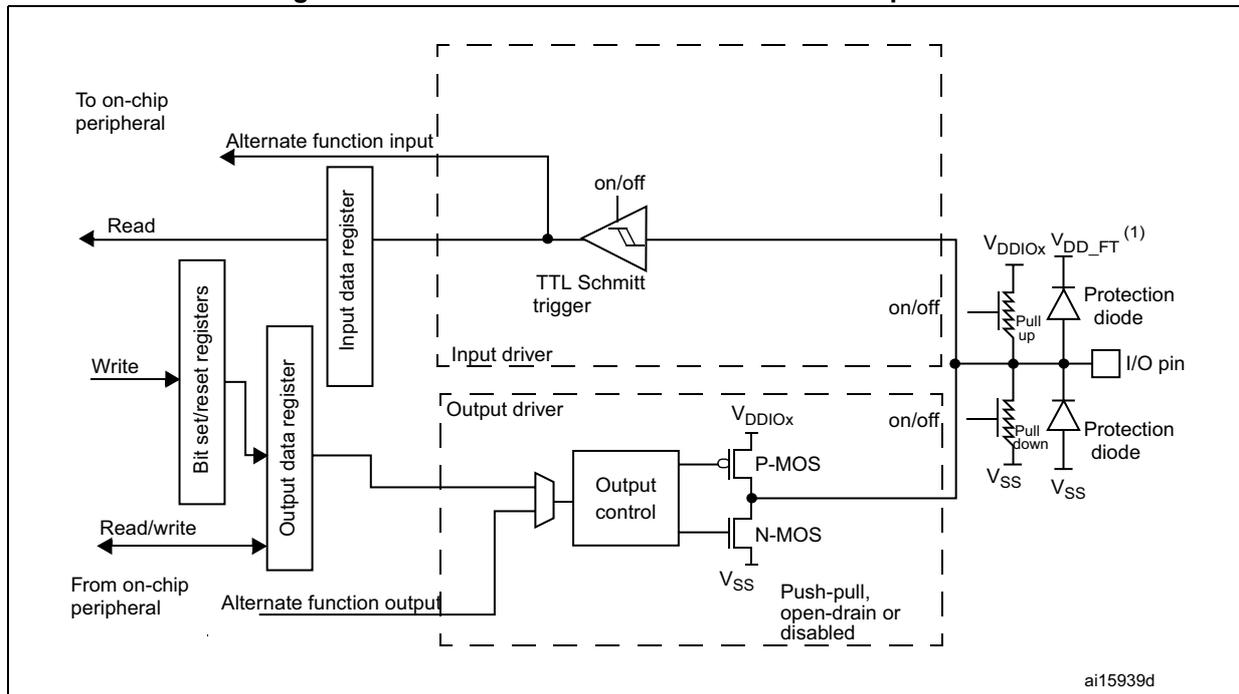
1.  $V_{DD\_FT}$  is a potential specific to 5-Volt tolerant I/Os and different from  $V_{DD}$ .
