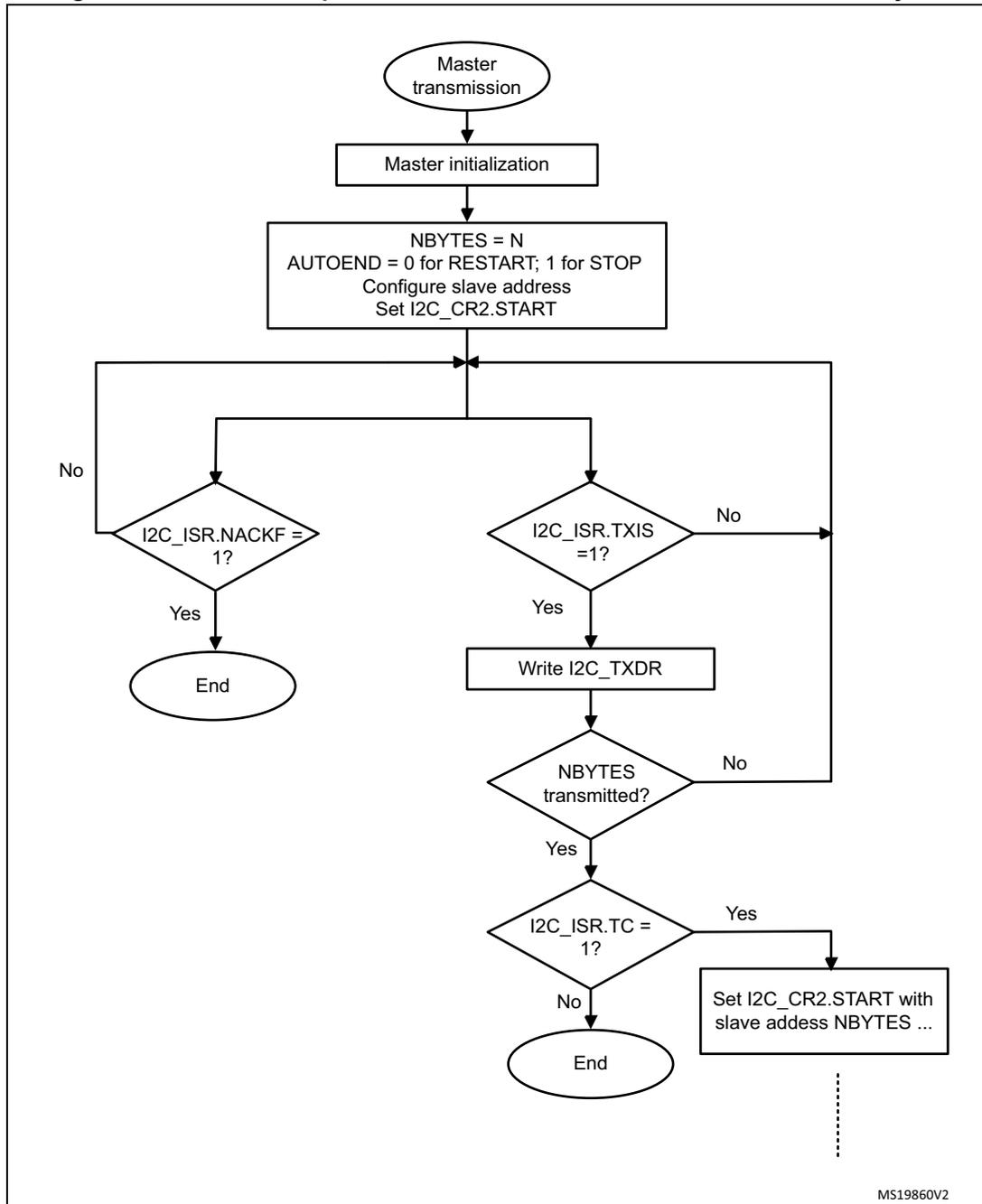
Figure 202. Transfer bus diagrams for I2C master transmitter
