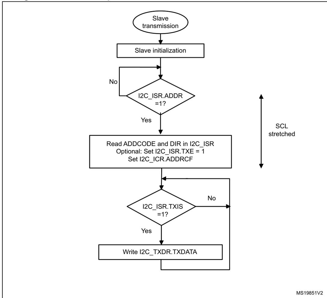
Figure 191. Transfer sequence flow for I2C slave transmitter, NOSTRETCH = 1
