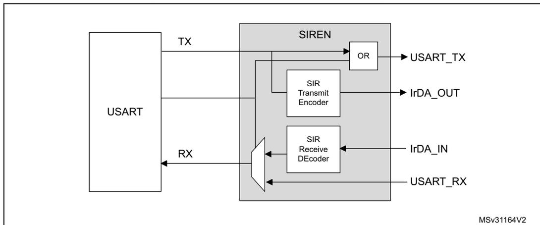
Figure 231. IrDA data modulation (3/16) -Normal Mode
