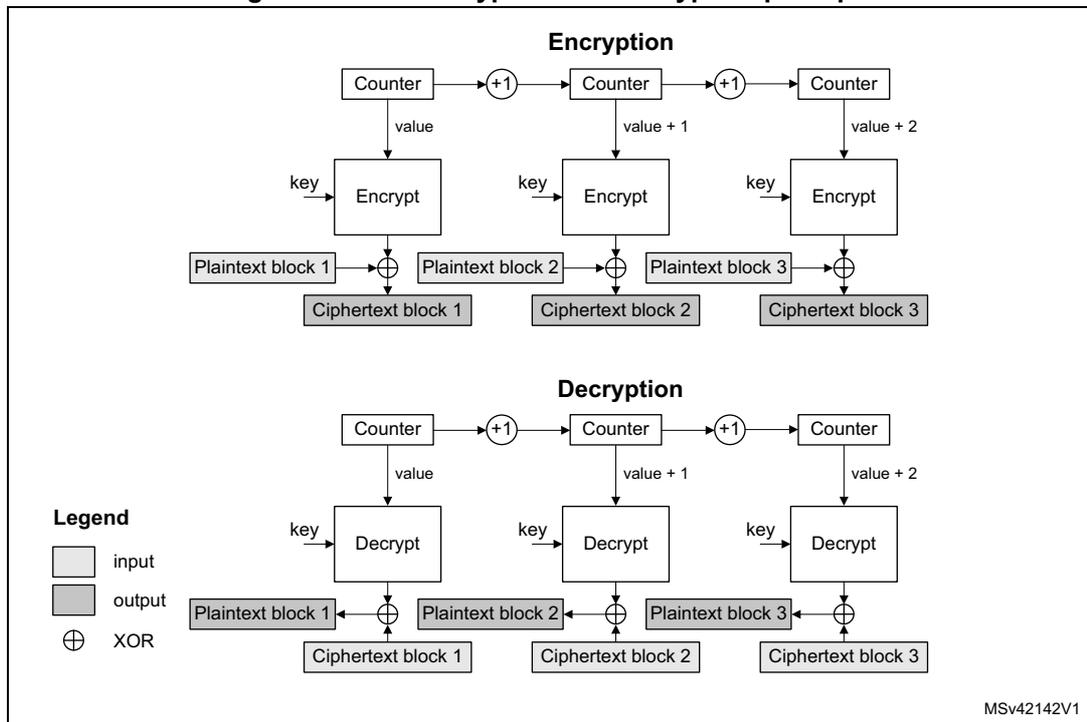
The CTR mode uses the AES core to generate a key stream. The keys are then XORed with the plaintext to obtain the ciphertext as specified in NIST *Special Publication 800-38A, Recommendation for Block Cipher Modes of Operation*.
