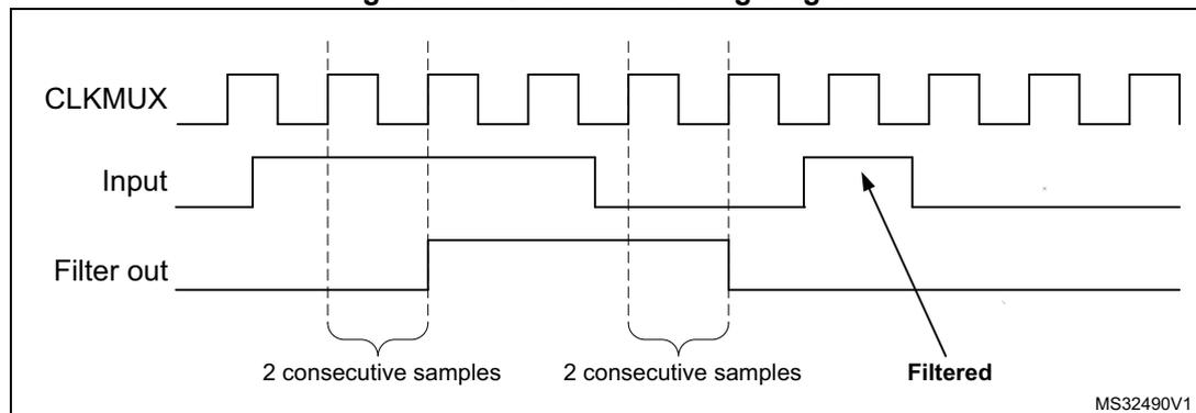
*Note:* In case no internal clock signal is provided, the digital filter must be deactivated by setting the CKFLT and TRGFLT bits to '0'. In that case, an external analog filter may be used to protect the LPTIM external inputs against glitches.
