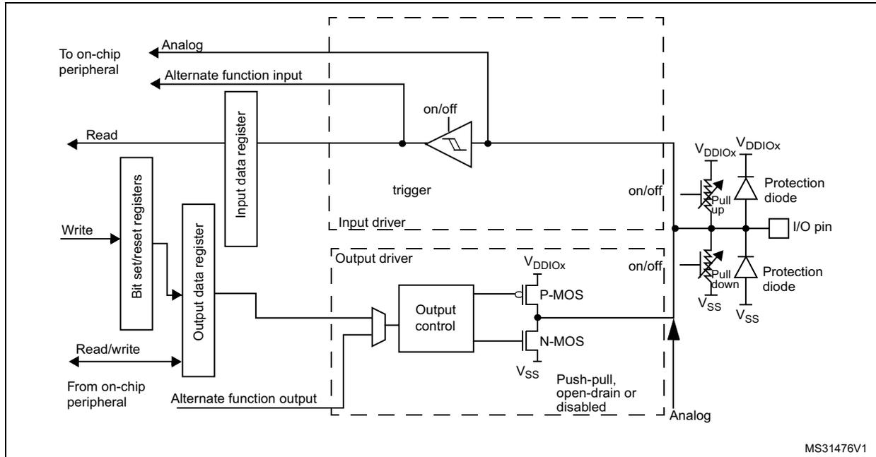
Figure 20. Basic structure of a 5-Volt tolerant I/O port bit
