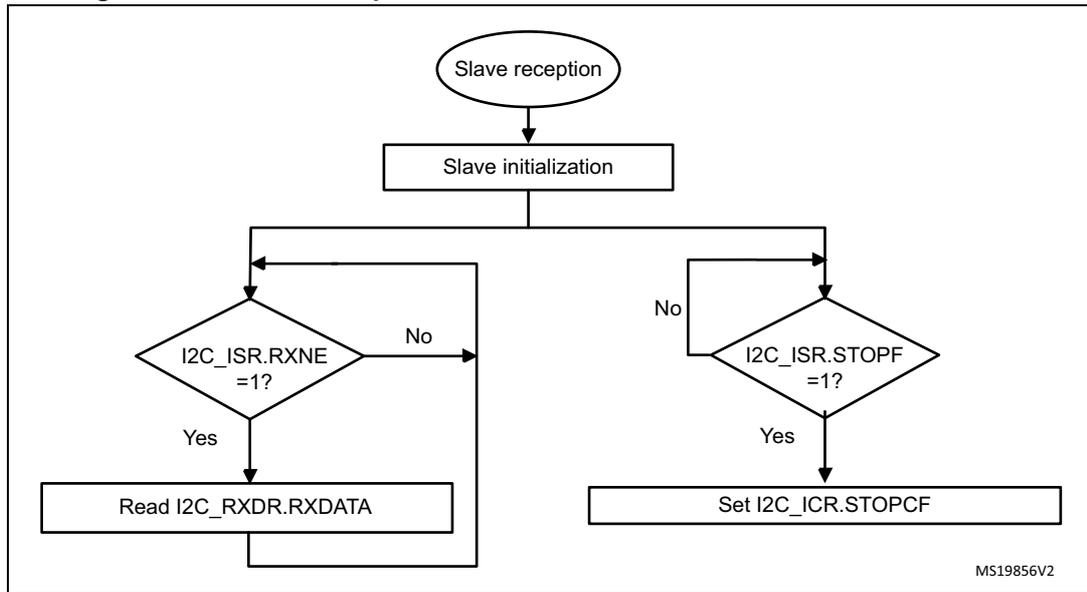
Figure 195. Transfer bus diagrams for I2C slave receiver
