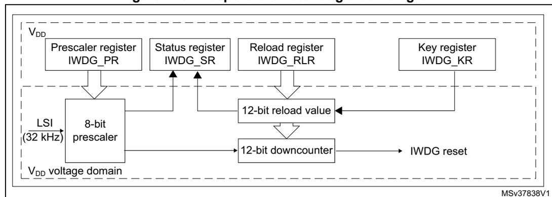
1. The register interface is located in the  $V_{DD}$  voltage domain. The watchdog function is located in the  $V_{DD}$  voltage domain, still functional in Standby mode.
