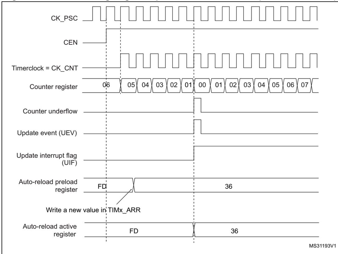
**Figure 141. Counter timing diagram, Update event with ARPE=1 (counter overflow)**
