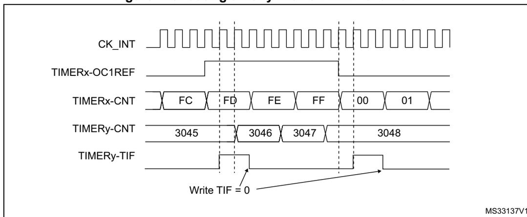
In the example in [Figure 118](#), the Timer y counter and prescaler are not initialized before being started. So they start counting from their current value. It is possible to start from a given value by resetting both timers before starting Timer x. Then any value can be written in the timer counters. The timers can easily be reset by software using the UG bit in the TIMx\_EGR registers.
