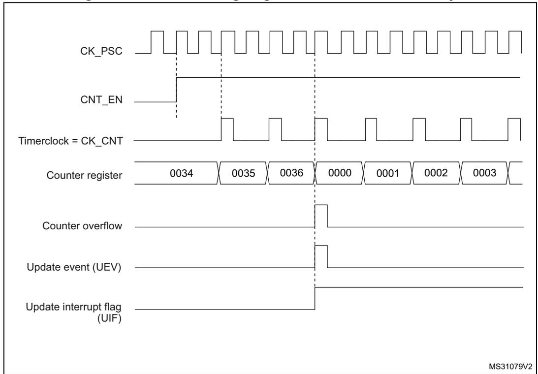
**Figure 128. Counter timing diagram, internal clock divided by 4**
