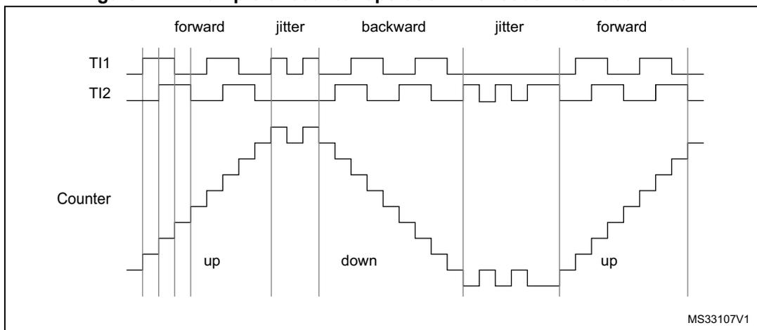
Figure 112 gives an example of counter behavior when TI1FP1 polarity is inverted (same configuration as above except CC1P=1).
