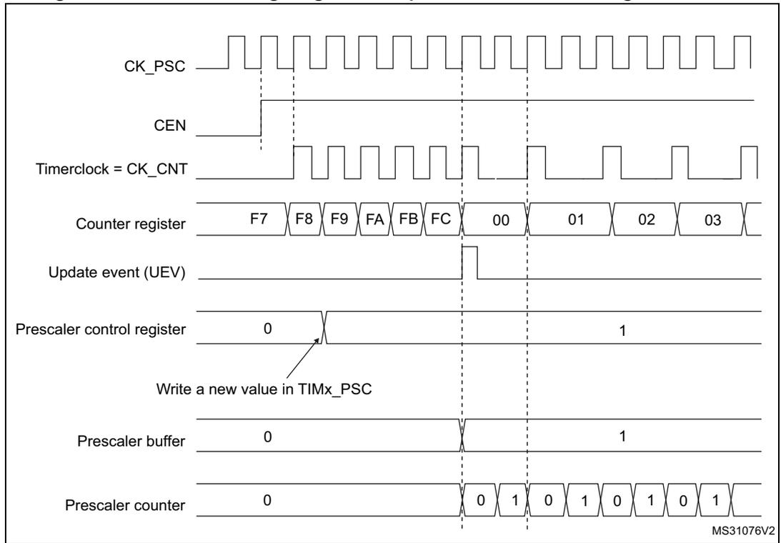
Figure 125. Counter timing diagram with prescaler division change from 1 to 4
