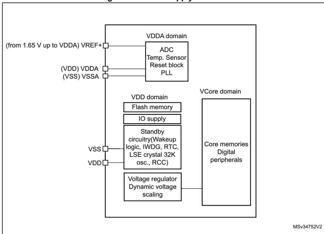
1.  $V_{DDA}$  and  $V_{SSA}$  must be connected to  $V_{DD}$  and  $V_{SS}$ , respectively.
