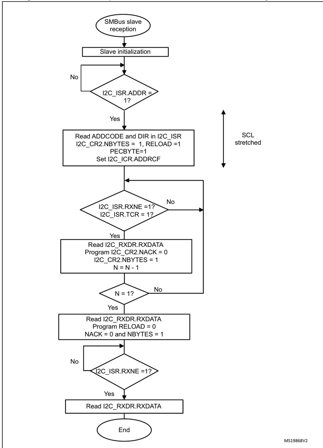
Figure 210. Bus transfer diagrams for SMBus slave receiver (SBC=1)
