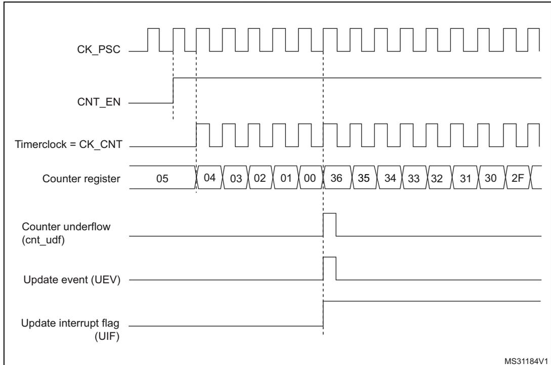
**Figure 87. Counter timing diagram, internal clock divided by 2**
