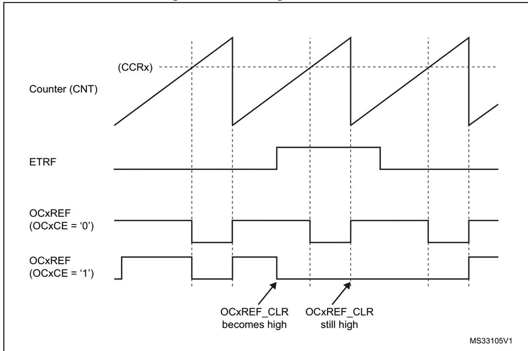
1. In case of a PWM with a 100% duty cycle (if  $CCR_x > ARR$ ), OCxREF is enabled again at the next counter overflow.
