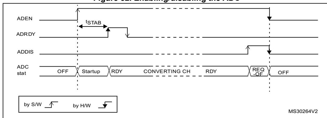
*Note:* In Auto-off mode (AUTOFF = 1) the power-on/off phases are performed automatically, by hardware and the ADRDY flag is not set.
