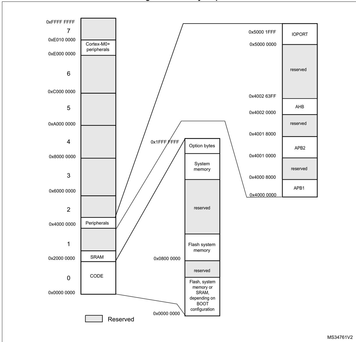
All the memory map areas that are not allocated to on-chip memories and peripherals are considered “Reserved”. For the detailed mapping of available memory and register areas, refer to the following table.
