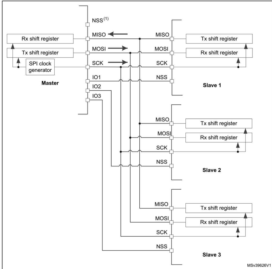
1. NSS pin is not used on master side at this configuration. It has to be managed internally (SSM=1, SSI=1) to prevent any MODF error.
