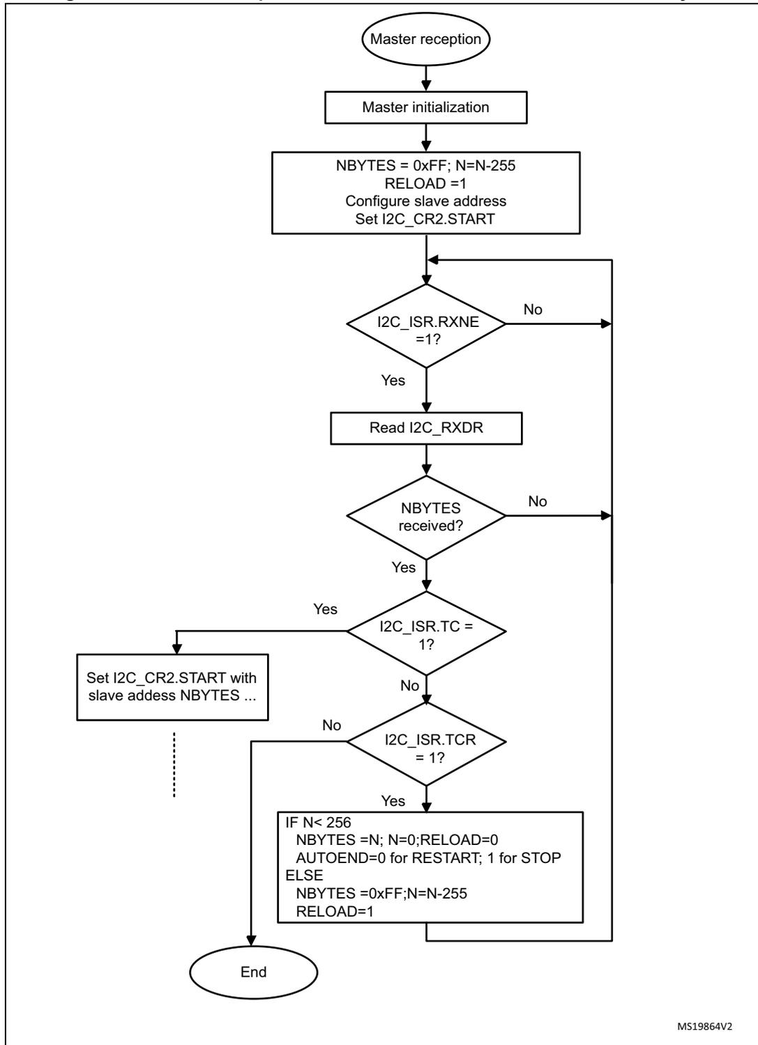
Figure 205. Transfer bus diagrams for I2C master receiver
