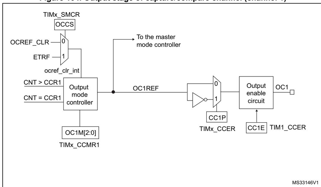
The capture/compare block is made of one preload register and one shadow register. Write and read always access the preload register.
